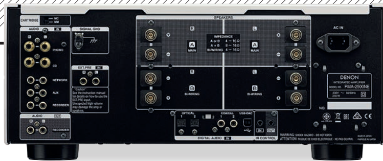
ABOVE: Three line, one tape in/out and MM/MC phono ins are joined by a preamp input and digital ins across S/PDIF (two optical, two coax) and asynchronous USB. Wired control is included and pairs of chunky 4mm speaker sockets assist bi-wiring
